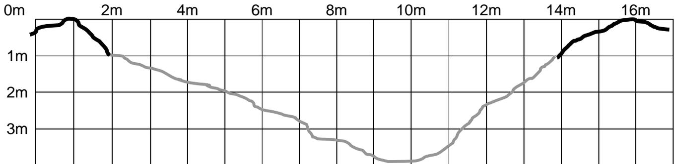
The cross section above represents cross section "A" with the addition of the stream banks. The top of the bank defines the maximum stream capacity. You have already calculated the cross section of the stream (# 1 above)
