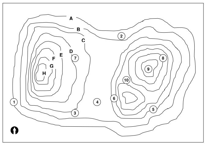
The **contour interval** for this map is **50m**. In the spaces below provide the correct elevation for each contour line, starting at the waters edge.
